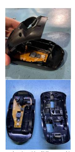
3. Remove the PCB from the mouse housing with a Philips screwdriver.
