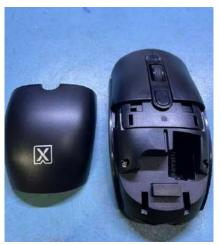
2. To locate the PCB. Remove the top cover with a Philips screwdriver.
