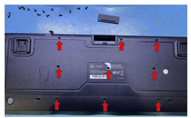
3. Separate the top cover from the rest of the keyboard
